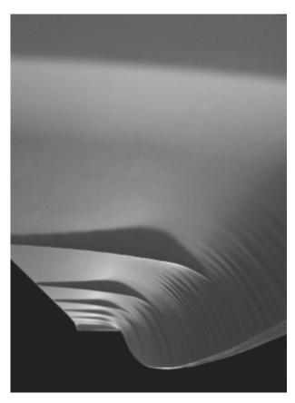
Figure 5. Plaster model of fabric-formed "Tee-beam"
